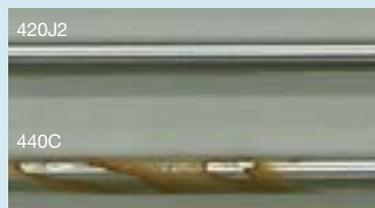
Immersion test in 5% saline solution for 24 hours
